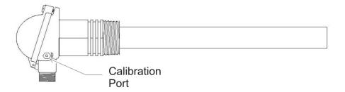
Figure 4-2: Calibration Port on Probe Head
